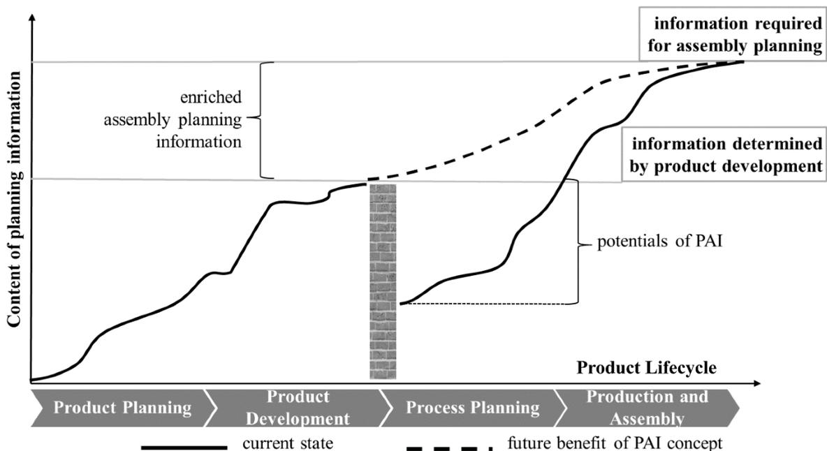
Figure 1. Information transfer along the Product Lifecycle is often disrupted by a systemic and methodically wall between Product Development and Process Planning (Eigner et al., 2013)
