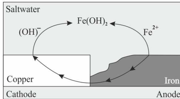
Figure 2. Corrosion process (Schulze, 2010)
