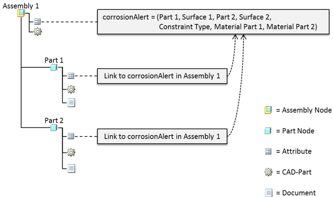
Figure 6. PDM Assembly Structure based on PTC Windchill
