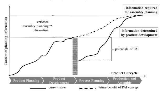
Figure 1. Information transfer along the Product Lifecycle is often disrupted by a systemic and methodically wall between Product Development and Process Planning (Eigner et al., 2013)
