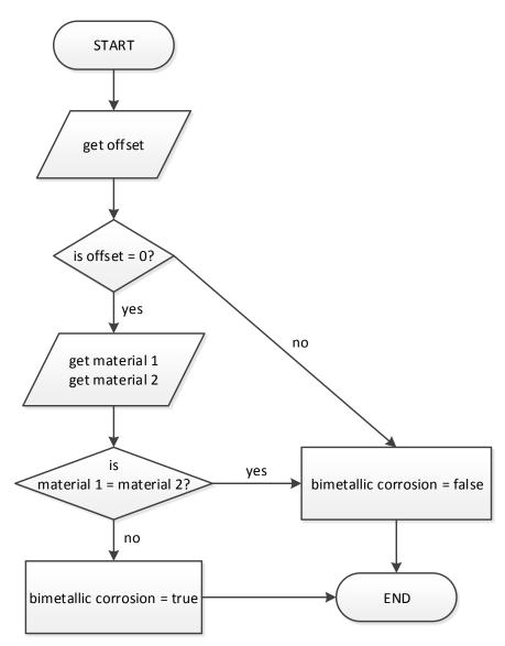
Figure 5. Flow chart of the detection procedure
