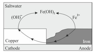
Figure 2. Corrosion process (Schulze, 2010)
