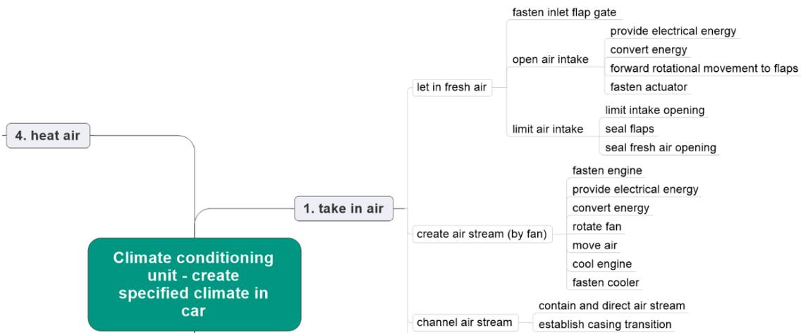
Figure 5. Function tree climate control unit
