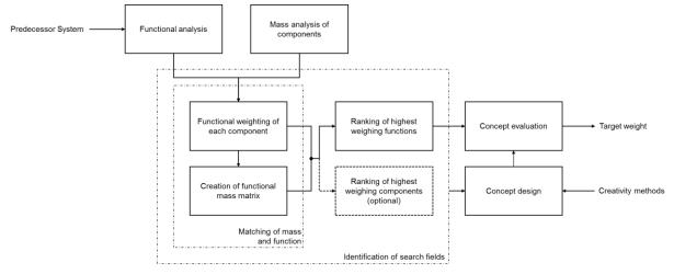
Figure 3. Target weighing process
