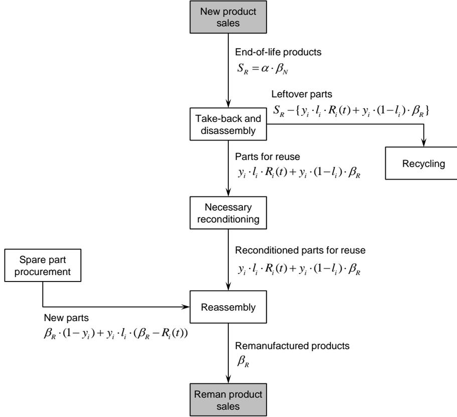
Figure 3. Remanufacturing process and product/part flow volumes
