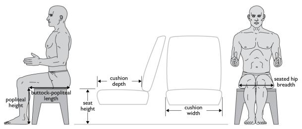
Figure 1 - The seat design parameters and their corresponding body dimensions.
