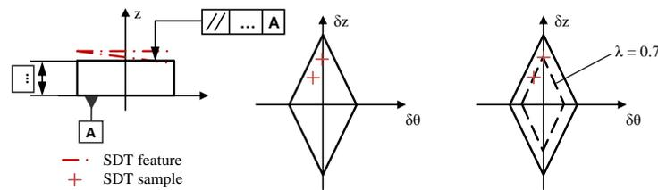
Figure 5. Deviation quality  $\lambda=0.7$  for two deviated planes in two dimensions with respect to a parallelism tolerance to datum A
