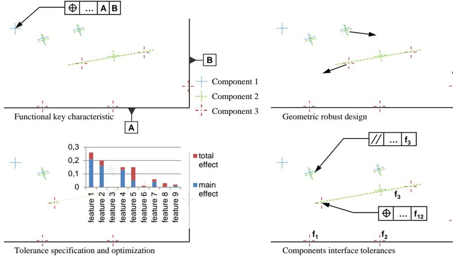
Figure 3. Skeleton model (upper left), robust design (u. r.), tolerance specification and optimization with contributors (l. l.) and final component interface tolerances (l. r.)
