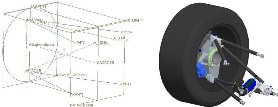
Figure 2. Skeleton model and volume model of a racing cars wheel suspension (Running snail racing team, RS 10)
