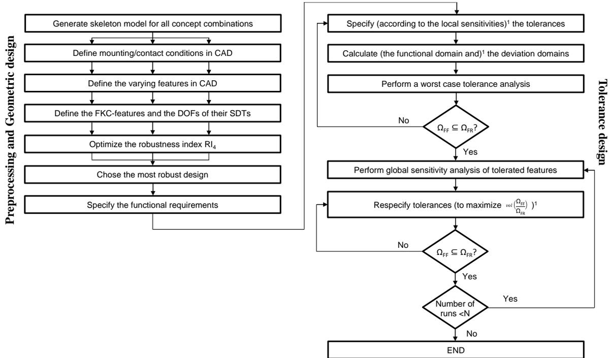
Figure 4. Scheme of the proposed tolerance management method, (...) <sup>1</sup> are notes for the first time the step is performed
