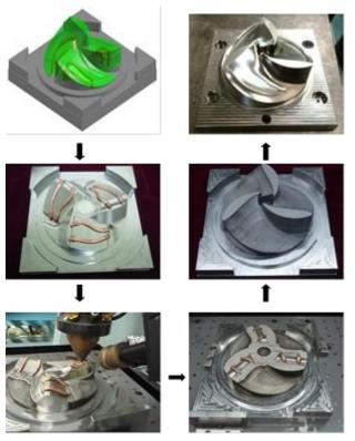
Figure 8. Conformal cooling channel made on a plastic injection mould die using DMT.
