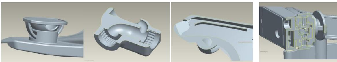
Figure 7. Examples of “designed for AM” features.
