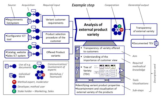
Figure 3. Developed notation to visualise steps of methods (as an example applied to one step of the Integrated PKT-approach)
