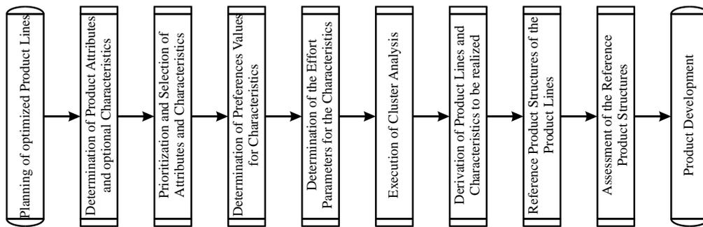
Figure 1. Steps of the methodology for planning of optimized product lines
