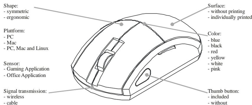
Figure 5. Computer mouse with seven attributes and 19 characteristics
