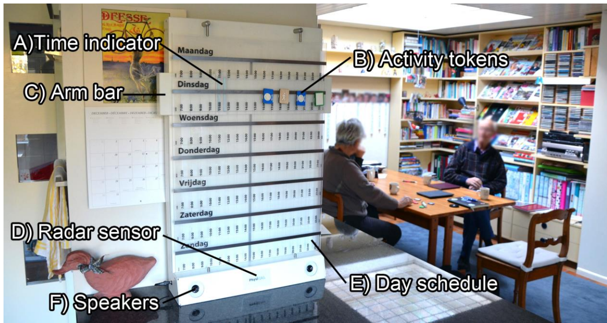
Figure 3. A picture of the PhysiCAL proposition being used in the home environment.
