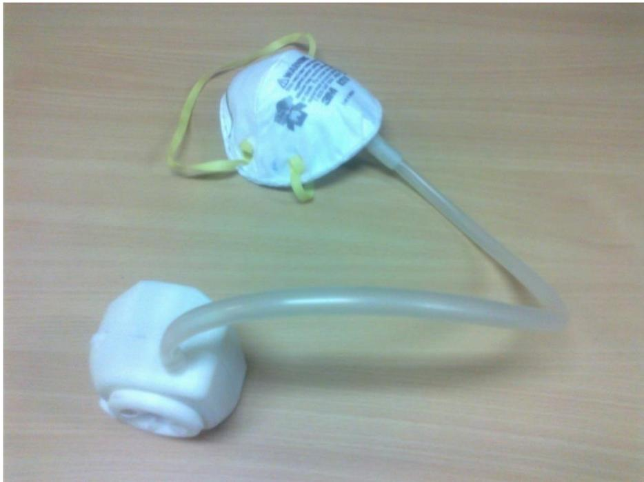
Figure 8. A refined working prototype
