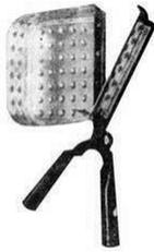
Figure 1. Manual tea plucking shears
