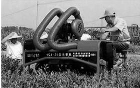
Figure 5. China made self-propelled automatic Tea plucking machine
