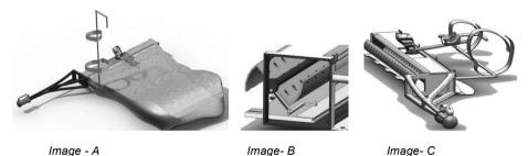
Figure 10. View of manual tea leaf plucking machine and tea collecting bag with flexible height adjustable support (Image-A), wiper fixed with fulcrum joint which is connected with plucking blades (Image-B) and ergonomic joystick like operating lever (Image-C)
