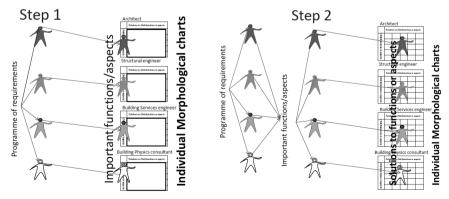
Figure 1. First two steps using the morphological charts in the Integral design method
