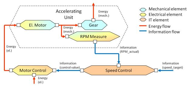
Figure 2: Exemplary active structure of an accelerating unit (representation according Gausemeier and Kahl (2010))
