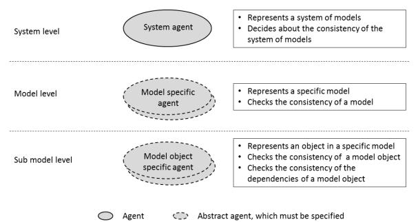
Figure 6: Architecture of the agent-based system
