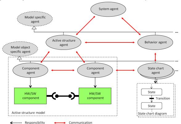
Figure 7: Exemplary agents for the active structure model and the behavior model
