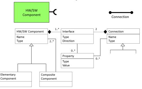
Figure 4: Extract of the class diagram for the meta model active structure
