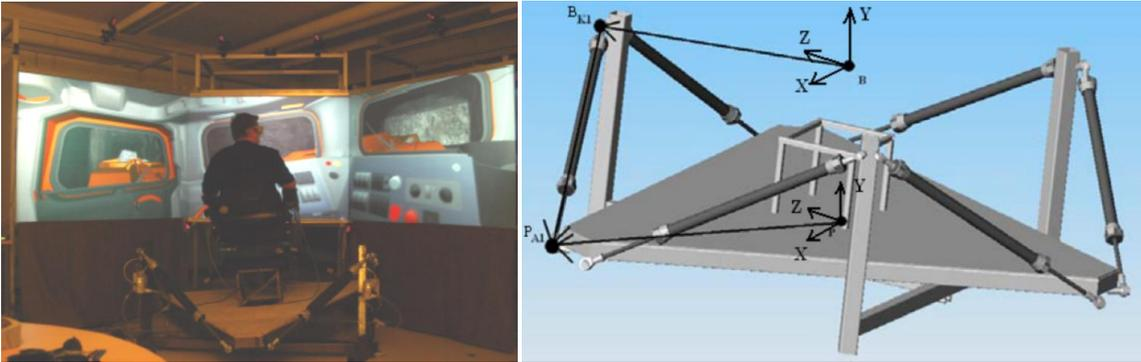
Figure 1. Virtual environment for vehicle testing and construction of motion platform
