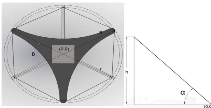
Figure 2. Structure and main parameters of an inverse Stewart-platform
