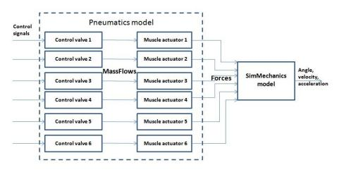
Figure 3. High-fidelity model in Matlab Simulink/SimMechanics
