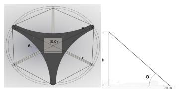
Figure 2. Structure and main parameters of an inverse Stewart-platform
