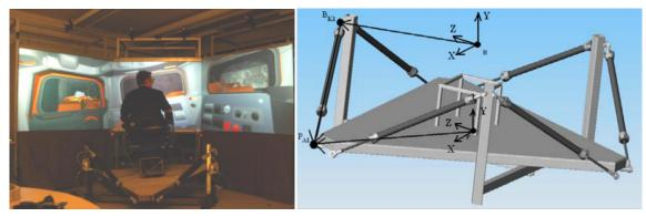
Figure 1. Virtual environment for vehicle testing and construction of motion platform
