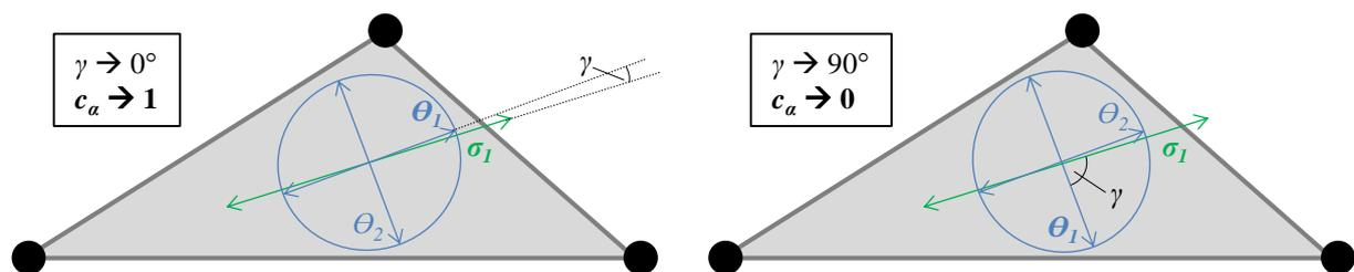
Figure 6. Angle criterion  $c_\alpha$  in case of almost isotropic fiber orientation
