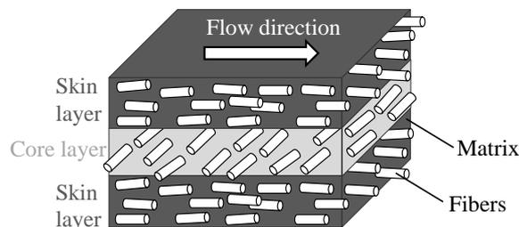
Figure 1. Three layer model of the cross section of a part made of SFRT
