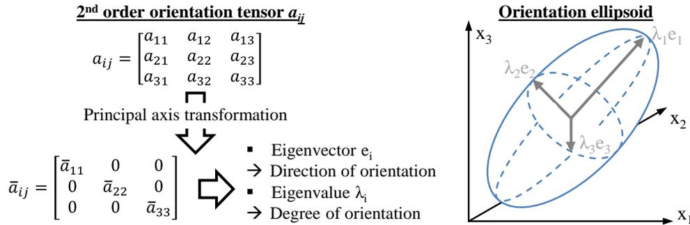
Figure 2. Fiber orientation condition described by the 2<sup>nd</sup> order orientation tensor  $a_{ij}$
