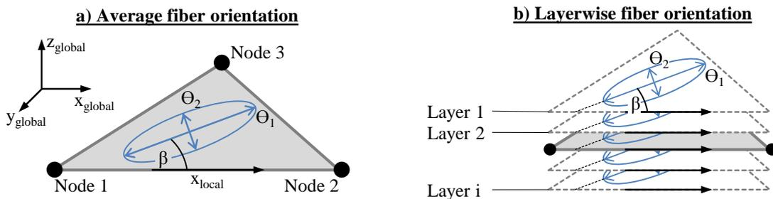
Figure 4. Fiber orientation in tria shell element
