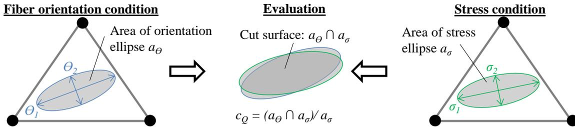
Figure 7. Determination of the overlap rate of stress and orientation ellipses
