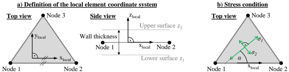
Figure 3. Local element coordinate system and stress trajectories in tria shell element
