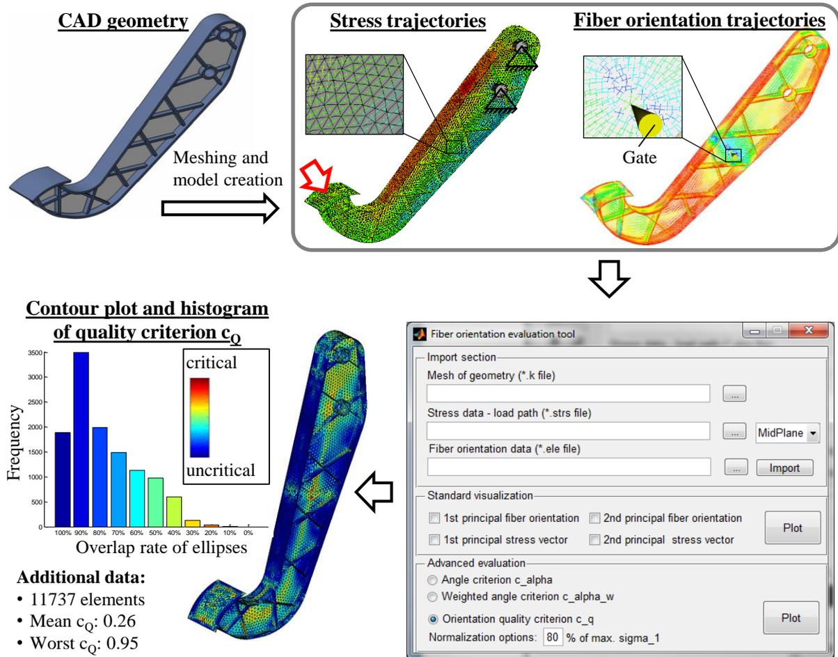
Figure 8. Workflow of the evaluation procedure
