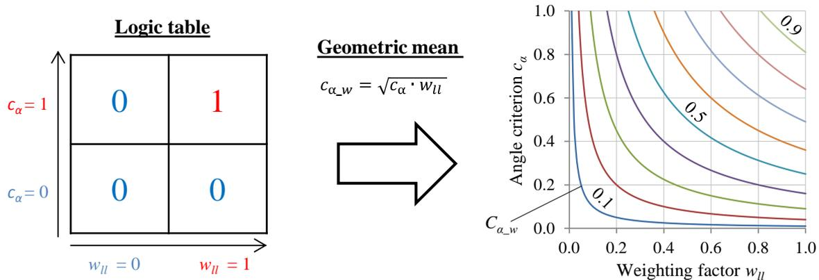
Figure 5. Weighting of the angle criterion  $c_\alpha$  with the load level factor  $w_{II}$
