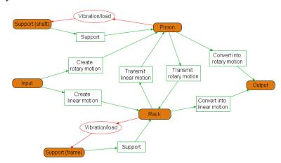
Figure 9 Example FAD for a rack and pinion
