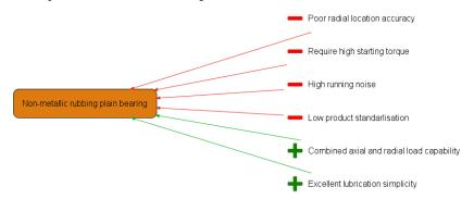
Figure 5 Example of advantage and disadvantage analysis of non-metallic rubbing plain bearing
