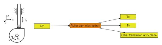
Figure 4 Movement analysis and attributes of a roller cam mechanism
