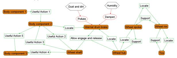
Figure 12 FAD of the wheel module of the sample robot
