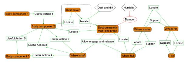
Figure 13 FAD of the final improvement Table 3 Comparison of brake actuation
