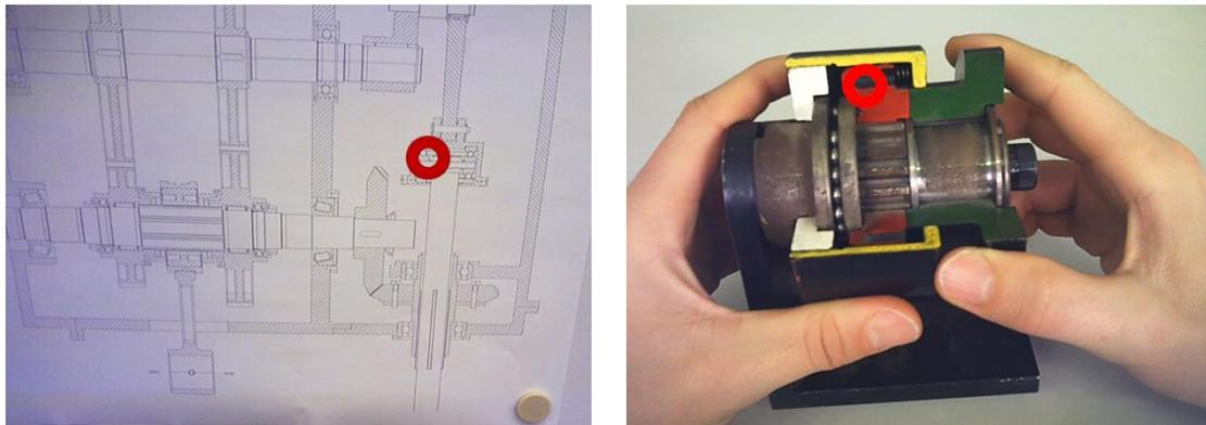
Figure 3. 2D sectional drawing (left) and demonstration model of a clutch (right) both with point of gaze marked with a red circle
