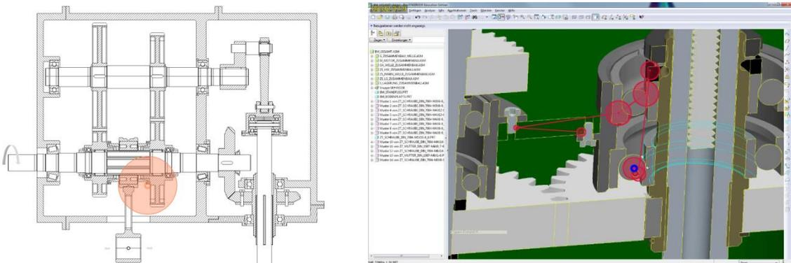
Figure 2. 2D sectional drawing with the actual fixation marked with an orange circle (left) and 3D CAD assembly with a scan path in red circles and lines (right)
