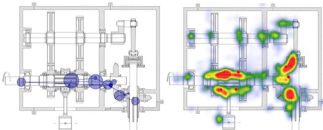
Figure 5. Scan path (left) and heat map (right) on a 2D sectional drawing
