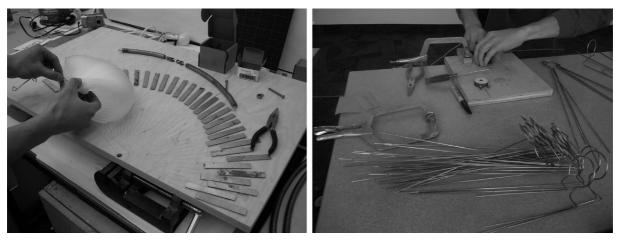
Figure 3. Student-made fixtures used for cutting sheet plastic and bending steel wire
