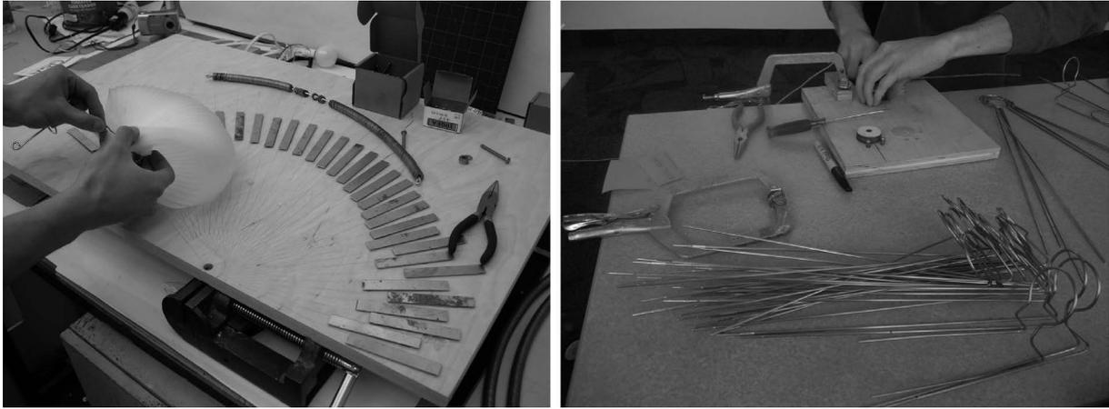
*Figure 3. Student-made fixtures used for cutting sheet plastic and bending steel wire*
