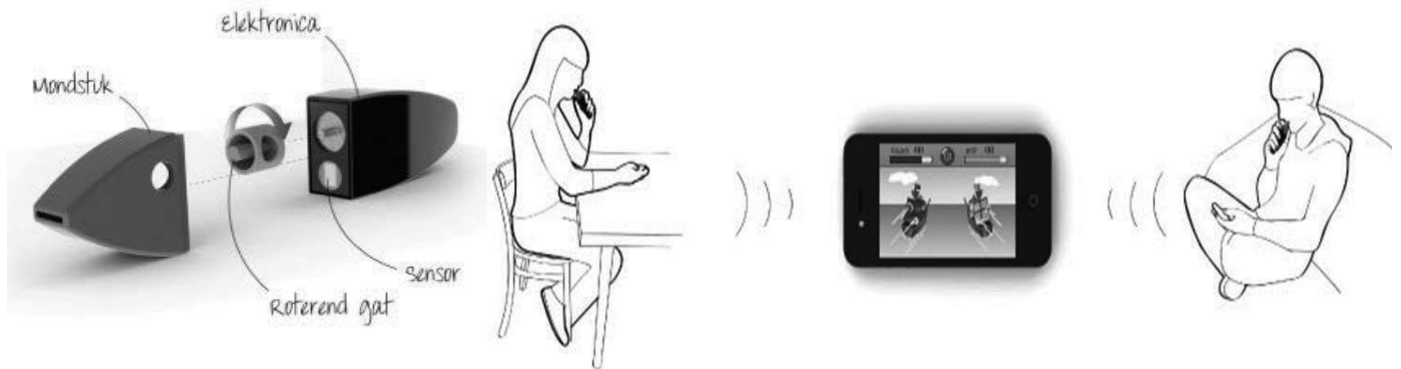
Figure 4. Movi: Left exploded view in 3 parts: mouthpiece, rotating opening and electronics; Right: drawing of a possible use situation, with ongoing “battle” on the handheld’s screen
