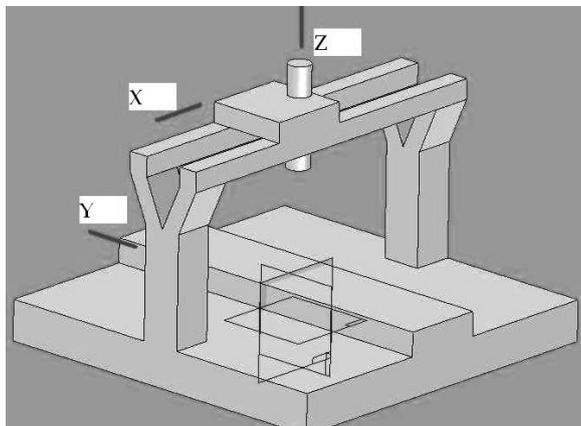
**Figure 2.** Conceptual workstation showing X-Y-Z slides.
