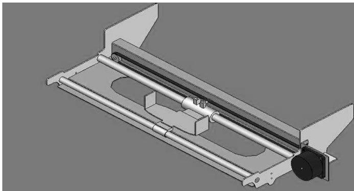
**Figure 3.** EPSON FX-100 dot matrix printer slide.
