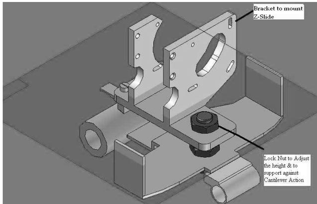
Figure 5. Modified slider of X-Slide.
