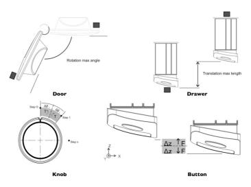
Figure 4. Implementation of the four haptic effects.
