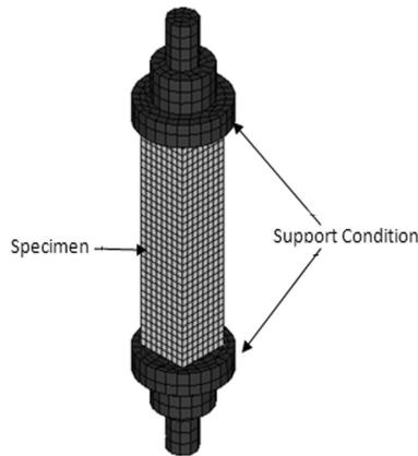
**Figure 2.** Three-dimensional finite element model.
