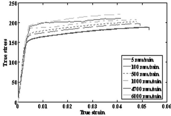
Figure 5. True Stress vs. True strain curve of aluminium used in the Study.
