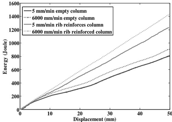
**Figure 12.** Energy vs. displacement curves for empty and rib reinforced box column for two different rates.
