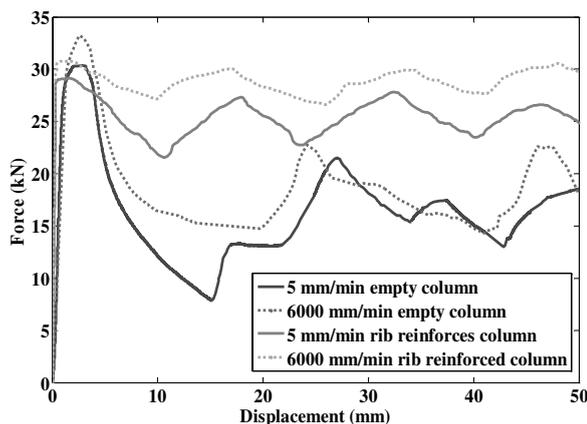
**Figure 8.** Force vs. displacement curves for empty and rib reinforced box column for two different rates.
