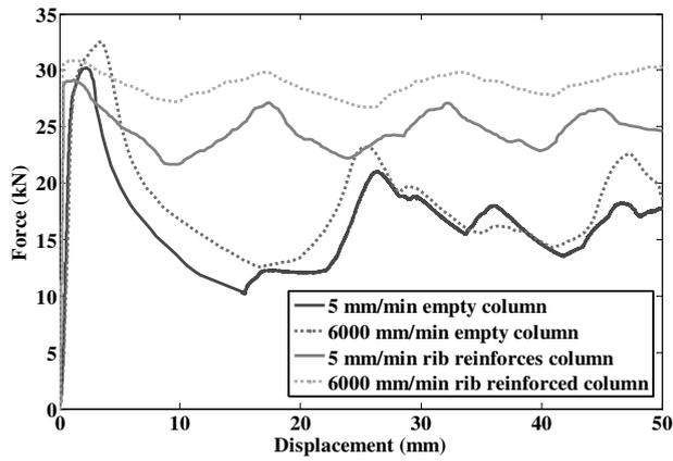
**Figure 11.** Force vs. displacement curves for empty and rib reinforced box column for two different rates.
