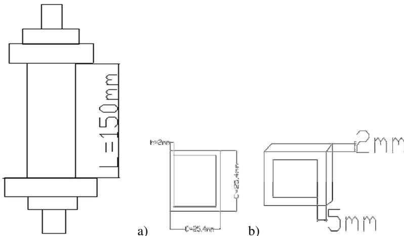
**Figure 1.** Geometry and support condition of structure. a) Empty extruded aluminum cross section. b) Rib geometry.
