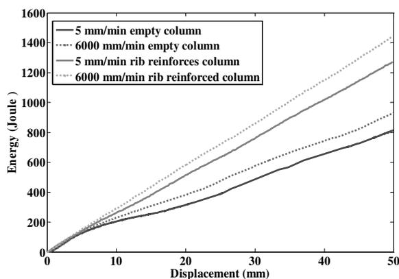
**Figure 9.** Energy vs. displacement curves for empty and rib reinforced box column for two different rates.
