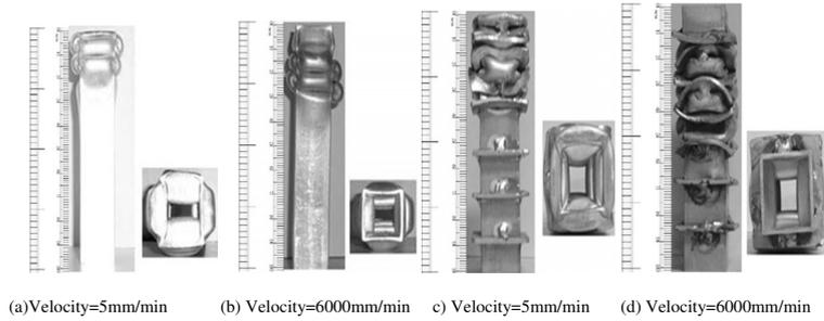
**Figure 10.** Collapse behaviour of empty and rib reinforced aluminum specimens obtained from experimental investigation when subjected to axial crushing at two different rates. (a) Velocity = 5mm/min (b) Velocity = 6000mm/min (c) Velocity = 5mm/min (d) Velocity = 6000mm/min
