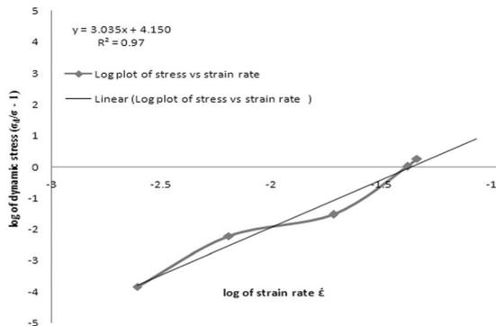
Figure 6. Log plot of stress vs. strain rate.
