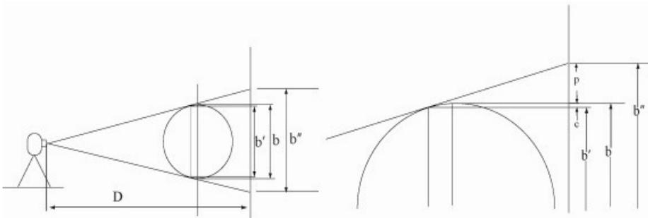
Figure 4. Parallax errors.
