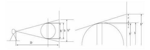
Figure 4. Parallax errors.
