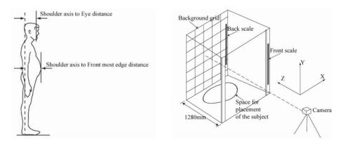
Figure 2. (a) Planar intra body dimensions, (b) Setup Schematic.
