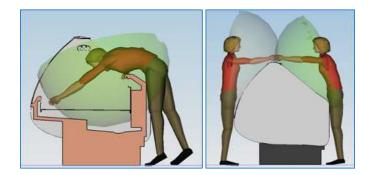
Figure 7. Postures for the horizontal serve-over display unit.
