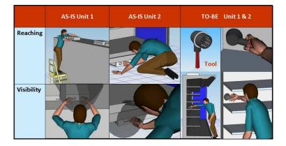
Figure 8. As-Is and To-Be configuration for electric equipment.
