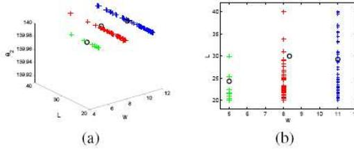
**Figure 5.** Design space with different standard sizes of  $w$  5, 8 and 11 cms. (a) Three clusters are shown in three colors in the design space  $w, L$  and  $\theta_2$  and the same clusters are shown in the design sub-space  $w, L$ .
