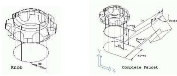
**Figure 2.** Complete Faucet with Knob. The driving parameter set  $\{W_o, H_o, L_o, \theta_1, \theta_2\}$  And the Knob radius  $\{R_b\}$  is  $0.5W_o$ .
