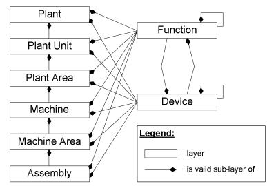
Figure 5. Layer configuration in electrical engineering framework of a plant (example) similar to the international standard ANSI/ISA-95
