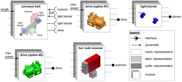
Figure 1. Module library for the conveyor belt containing the mandatory (*conveyor belt*) and optional (*drive*, *light barrier*, *bar code scanner*) basic modules with their discipline representations
