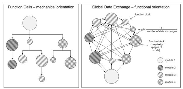
Figure 4. Schematic diagram of differences between mechanical-structured function calls and functional-structured data exchange
