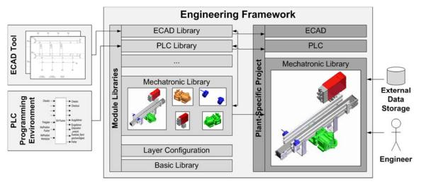
Figure 6. Exemplary information flow and data storage in an engineering framework
