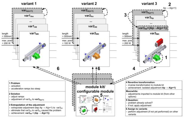
Figure 2. Variant management and tracing of changes for the conveyor belt
