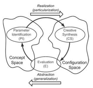
Figure 1. The 3-step prescriptive model of parameter analysis drawn on top of the 2-space descriptive model
