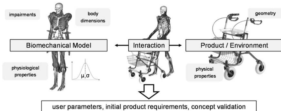
**Figure 5. Biomechanical simulation**
