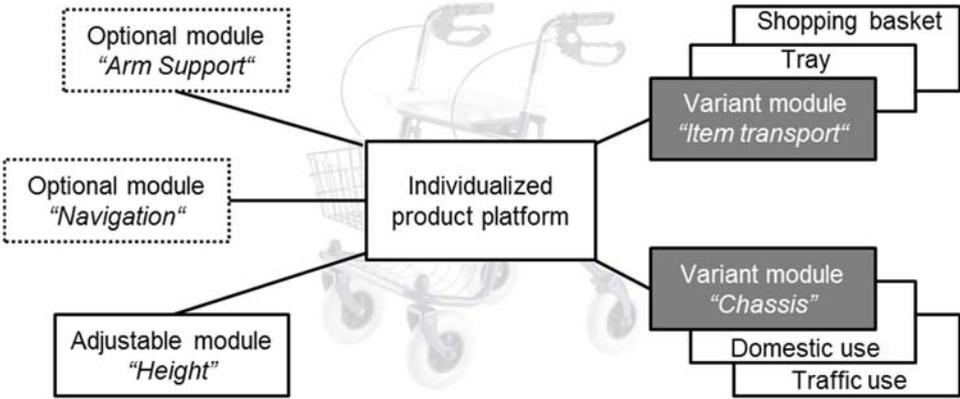
**Figure 7. Example for configuration of a user-specific variant walking frame**
