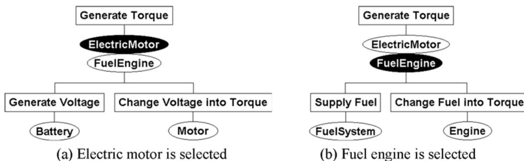
Figure 1. Examples of function / means tree
