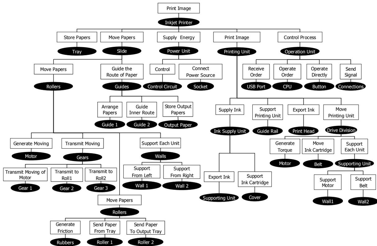
Figure 8. F/M tree of an inkjet printer
