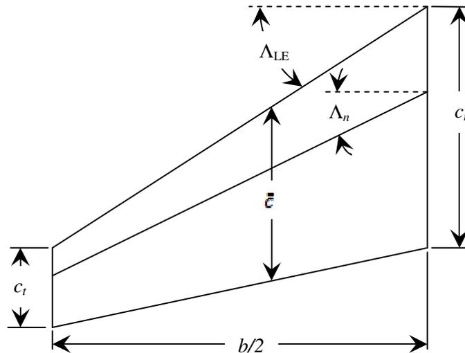
Figure 1. Wing geometry used in robust design assignment, based on Ref. 13
