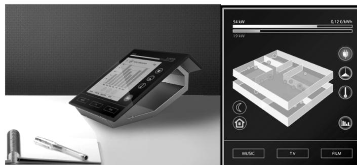
Figure 2. Echo – a household energy control device and its interface
