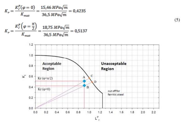
Figure 5. Assessment points using API RP 579 code
