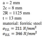
Figure 2. Pipe geometry and its mechanical properties
