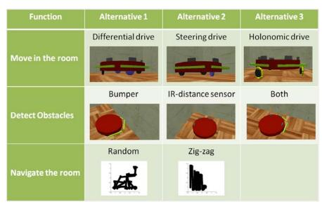
Figure 2: Zwicky matrix of the possible vacuum cleaner concepts
