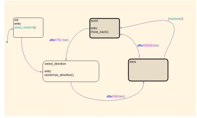
Figure 4: The FSM implementation of the robot's random navigation algorithm
