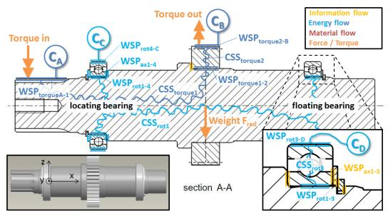
Figure 8: C&C-A analysis of a simplified gearbox input shaft
