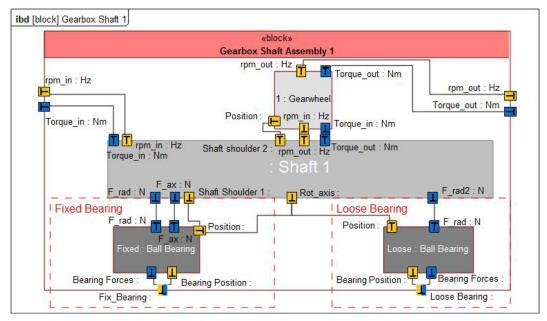
Figure 9: Gearbox input shaft modeled in C&C-M for SysML
