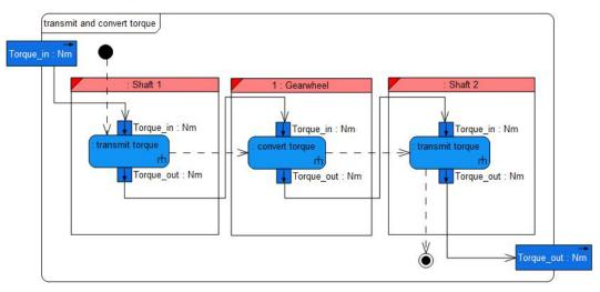
Figure 11: Function decomposition "transmit and convert torque"
