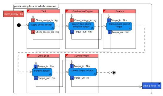
Figure 10: Function decomposition "provide driving force for vehicle movement" in a SysMLactivity diagram
