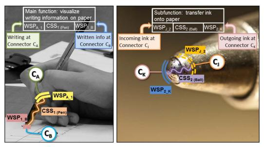
Figure 2: C&C-A description of the process of writing with a ball pen [17]
