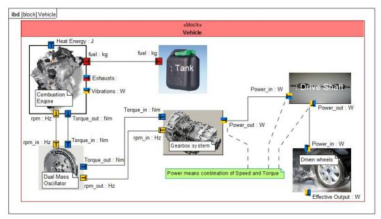
Figure 7: Internal Block Diagram of the exemplified vehicle assembly
