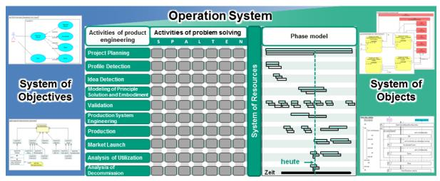
Figure 1: The integrated Product engineering Model (iPeM)
