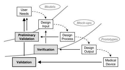
Figure 4. Simplified Waterfall Model with successive use of models, mock-ups and prototypes during the design process and the verification and validation steps; models and mock-ups can serve in a preliminary validation at the end of the conceptual design (adapted from [2])
