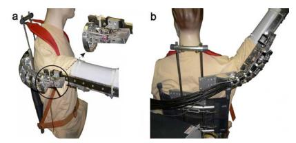
Figure 6. Shoulder module of the 6 DOF exoskeleton in (a) antepulsion and (b) abduction movements
