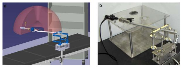
Figure 8. (a) Virtual model and (b) passive mock-up of the active laparoscope positioner
