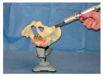
Figure 3. Plastic model of bone used for experimental quantification of cutting accuracy [12]
