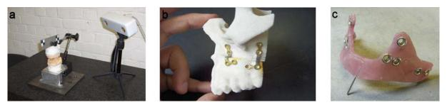
Figure 2. Verification mock-ups and prototypes of the novel solution after reestablishment of patients and surgeons needs: (a) localization device to measure the required bone displacements, (b) rapid prototyping full-size model of the desired displacement after CT-scan based simulation, and (c) template to guide gestures during procedure.
