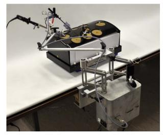
Figure 9. Proof of concept prototype of the laparoscope positioner
