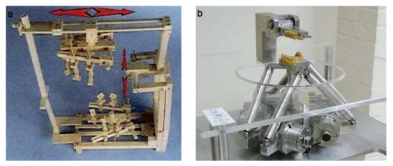
Figure 1. (a) Initial wood mock-up of maxillofacial robot presented by the surgeon [1] and (b) prototype of the solution proposed by the engineering team
