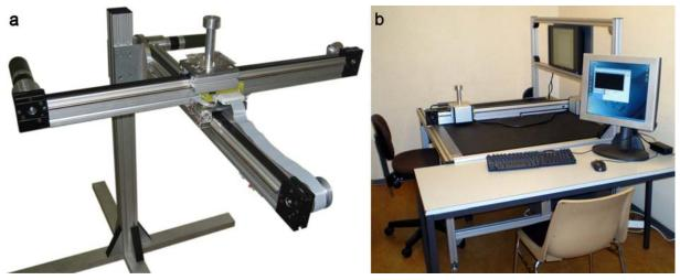
Figure 5. Evolution of the planar robot developed to prove the efficiency of the control scheme that ensures active compliance during manual manipulation: (a) initial partial mock-up and (b) detailed functional prototype
