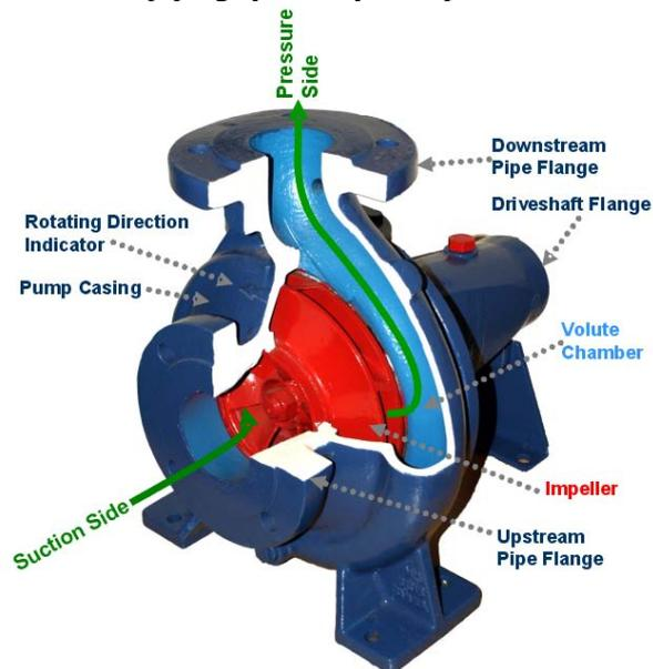
Figure 3: cross-section of a centrifugal pump, cit: Wasserwerk Delmenhorst
