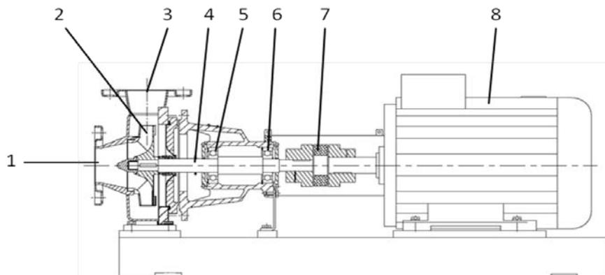
Figure 4. Sketch of the sample centrifugal pump [18]
