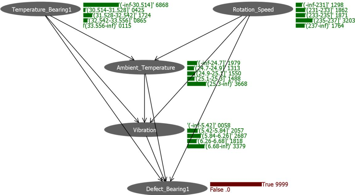
Figure 8. What-If-analyses for the defect of bearing 1
