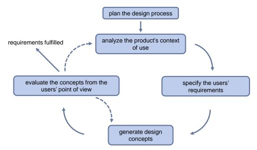
Figure 1. Human-centered design process according to EN ISO 9241-210
