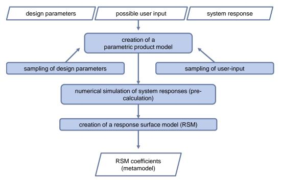
Figure 2. Process of model preparation
