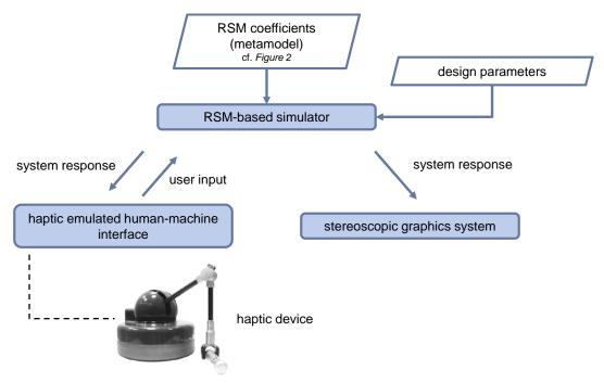
Figure 3. Topology of the simulation system
