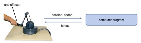
Figure 4. The haptic device and computer interface
