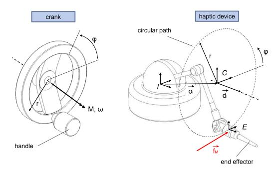
Figure 7. Emulation of a mechanical crank
