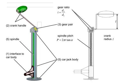
Figure 9. The Car jack and its crucial design parameters
