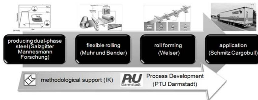
Figure 1. Schematic representation of the HIPAT process chain
