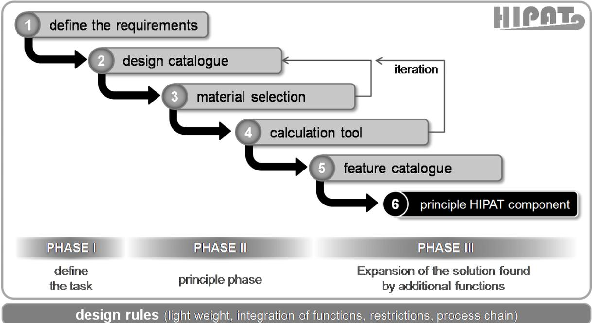
Figure 5. Schematic representation of the construction methodology for determining the basic shape of a HIPAT-component
