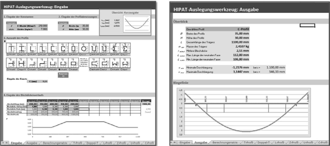
Figure 8. Input and output views of the user interface of the calculation tool, which helps the designer to refine the sheet thickness of the basic HIPAT profile
