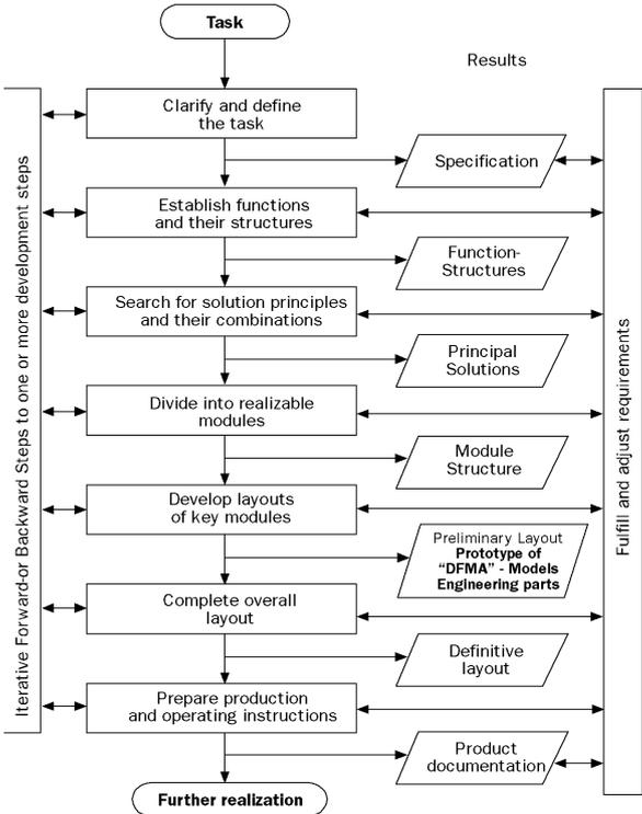
Figure 2. Process model VDI 2221 for the Systematic approach to the development and design of technical systems and products [4]
