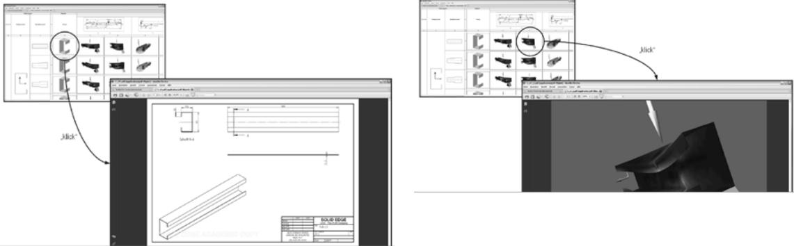
Figure 7. Example of a selected HIPAT profile or a load path in the interactive design catalogue and opening the production drawing of the component with the precise geometry or the 3D-pdf of the component
