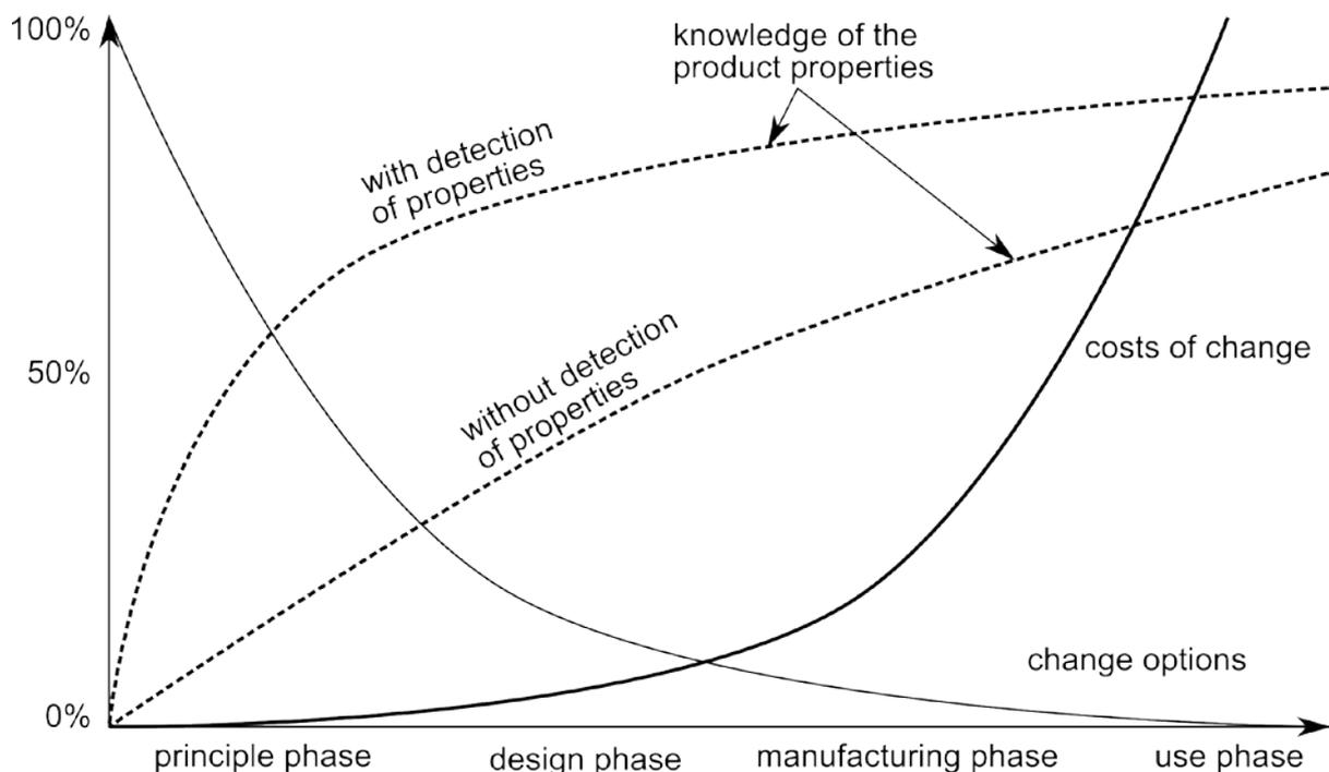
Figure 4. Schematic representation of the knowledge about the product characteristics with and without property detection during the product development process and highlight the options for change and the resulting change in cost [according to 10]
