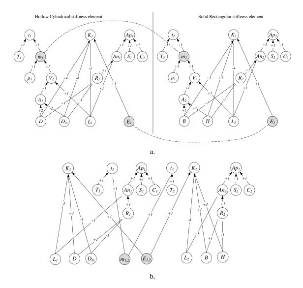
Figure 3. Redundancy eliminations and new common AWD: a. thirty two (32) DPs represented in two separate AWDs, b. twenty four (24) DPs represented in a common AWD
