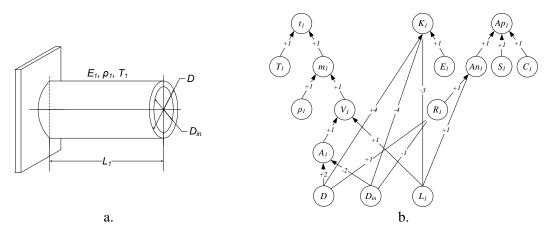
Figure 2. An alternative for a structural element: a. Cantilever beam of circular hollow section, b. AWD of design parameters.
