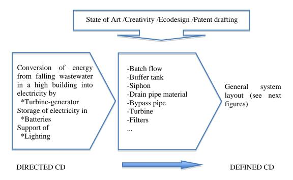
Figure 4. Process from directed conceptual design to defined conceptual design using creativity, Ecodesign and patent drafting tools of the case study.
