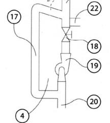
Figure 5. Diagram of the wastewater energy recovery system from a high building (1) with a buffer tank (2) and an electric system for illumination. Below is a drawing of the turbine system (4) with a turbine (19) and a bypass pipe (17).
