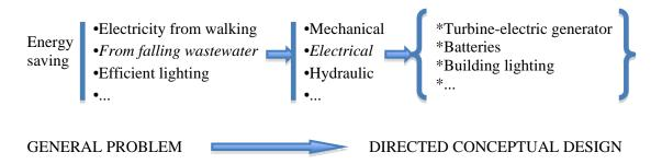
Figure 3. Process from general problem of energy saving in buildings to a directed conceptual design. The recovery of energy from falling wastewater by a turbine-electric generator was selected.
