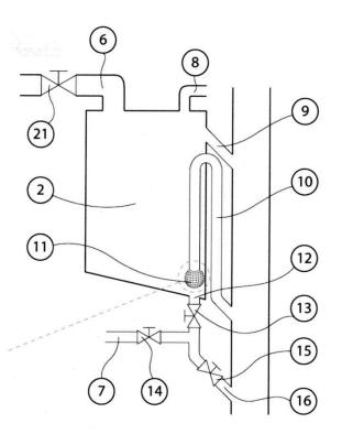
Figure 6. Diagram of buffer tank with automatic discharge by self-siphoning.
