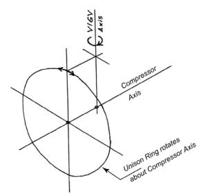
Figure 2. Schematic Diagram of Motion Requirements..
