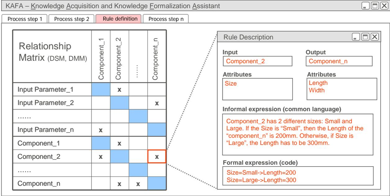
Figure 6. Concept View of KAFA (Knowledge acquisition and knowledge formalization Assistant) with extended knowledge object in DSM.
