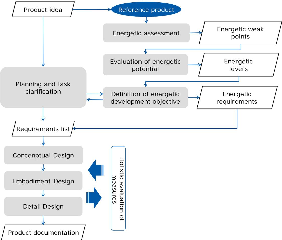
Figure 3: Energy efficient products – a design approach
