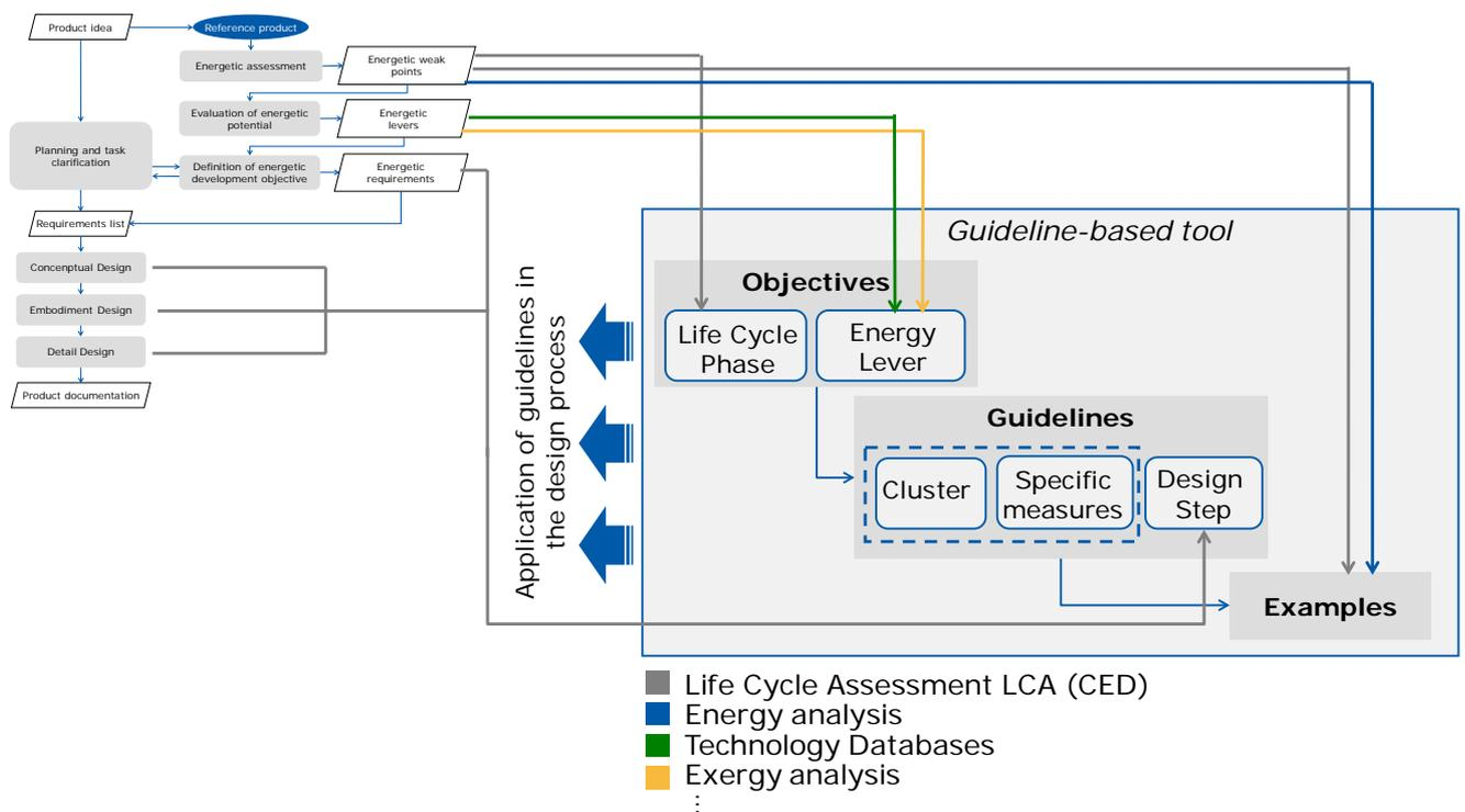
Figure 4: Integration of the guideline-based tool into the design approach
